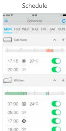
Schedule the set temperature, operation mode and fan speed
