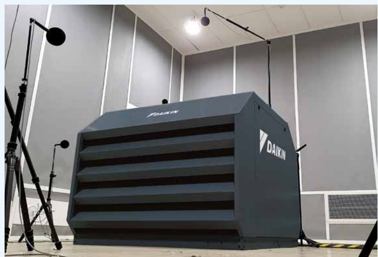
Sound power level measurement in acoustic chamber
